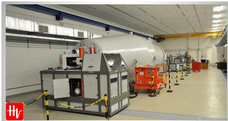
Fig. 1. The 6.0 MV coaxial High-Current Tandetron™ Cockroft-Walton- type accelerator at the Advanced Technologies Research Institute (ATRI) of the Faculty of Material Science and Technology of the Slovak University of Technology in Trnava, Slovakia.
