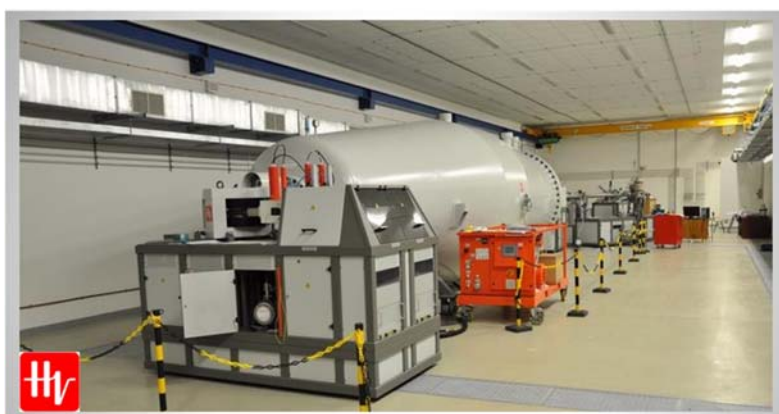
Fig. 1. The 6.0 MV coaxial High-Current Tandatron™ Cockroft-Walton type accelerator at the Advanced Technologies Research Institute (ATRI) of the Faculty of Material Science and Technology of the Slovak University of Technology in Trnava, Slovakia.
