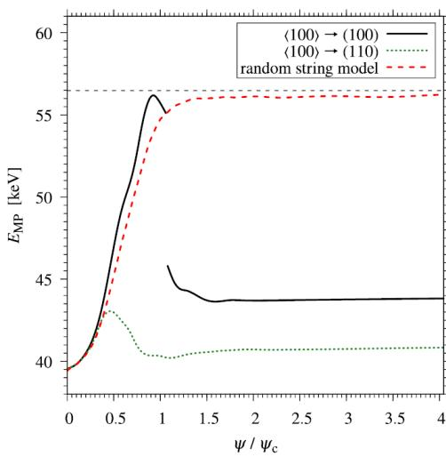
Dependence of the most probable energy loss of 3 GeV positrons in a silicon crystal of 200  $\mu\text{m}$  thickness on the angle between the incident particle momentum and the  $\langle 100 \rangle$  crystal axis. Dashed horizontal line –  $E_{MP}$  for a non-oriented crystal.
