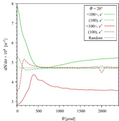
Dependence of the angular density of the number of CXR photons emitted from the upstream surface of the crystal on the angle between the atomic axis/plane and the momentum of the 1 GeV particles incident on the crystal.
